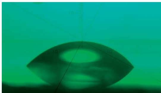
Figure 1 (online colour at: www.pss-rapid.com ) Contact angle measurement against pure water at pH of 5.5 at room temperature after dipping in amine solution for 4 h.
